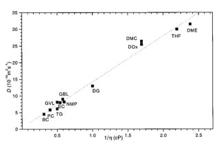
**Fig. 3** The relationship between the diffusion coefficient and viscosity of 12 organic solvents. Reproduced with permission from ref. 35, Copyright (1999). American Chemical Society.
