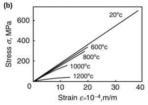
Fig. 4 (a) Illustration of the stress-strain relationship for brittle ceramics: ZTA and Y-PSZ have a brittleness measure of 1, whereas Syalon + BN and Mg-PSZ have a brittleness measure of 0.70 and 0.44, respectively. (b) The stress-strain relationship for Y-PSZ ceramics at different temperatures. Reproduced from ref. 50, Copyright (2014), with permission from Springer.
