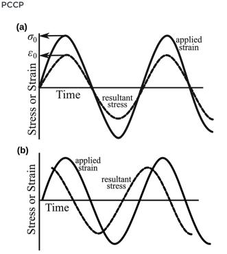
Fig. 9 Sinusoidal applied strain and the resultant stress response observed in (a) an elastic material and (b) a viscoelastic material. Reproduced with permission from ref. 56, Copyright (2012), Princeton University Press.
