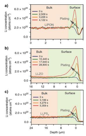
Fig. 10 Measurement of Li concentration profiles using operando neutron depth profiling technique across (a) LiPON (b) c-LLZO and (c) Li<sub>3</sub>PS<sub>4</sub> solid electrolytes. Reproduced from ref. 74, Copyright (2019), with permission from Springer Nature.
