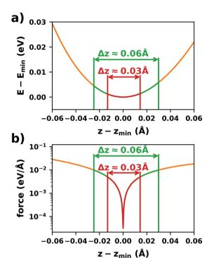
Fig. 19 (a) Total energy (relative to the minimum) of PTCDA on Ag(111) (calculated with PBE+vdW surf for a single molecule in a 6  $\times$  6 unit cell, as described in detail in Hörmann et al.)<sup>282</sup> as a function of its distance (relative to the equilibrium distance). (b) Force per atom acting on the PTCDA molecule in z-direction.
