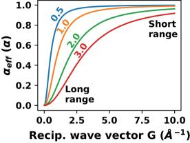
**Fig. 15** Effective mixing parameter  $\alpha_{\rm eff}$  as a function of the reciprocal wave vector G for different values of  $q_0$  when applying the Kerker preconditioner.
