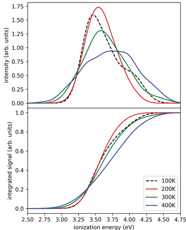
Fig. 3 Simulated ionization probabilities (upper panel) and their integral (lower panel) for  $\text{Na}(\text{H}_2\text{O})_7$  at different temperatures. The ionization probabilities are linked to the temperature dependent degree of sodium solvation. At low energies ion pairs are found, at high energies the sodium atom remains intact.
