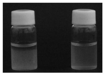
Fig. 1 Suspension of untreated cellulose nanowhiskers in water added with 1 M NaCl (left) and cellulose nanowhiskers after oxidation over a silica gelsupported TEMPO catalyst (right). [Reproduced from ref. 13, with kind permission].
