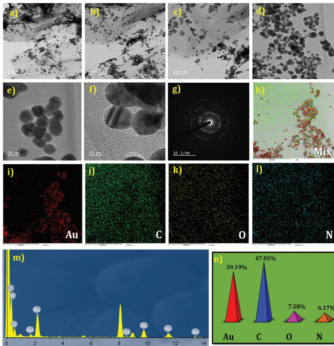
**Fig. 4** TEM images of AuNP/PEI/rGO at various magnifications (a–e). HRTEM (f) and SAED (g) patterns of AuNPs in the nanocomposite. Elemental mapping results of the AuNP/PEI/rGO nanocomposite (mixture) in (h) the presence of different elements including Au (i), C (j), O (k), and N (l). EDX result (m) and the corresponding weight percentage plot (n).
