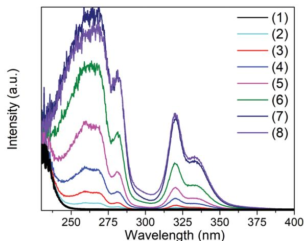
**Fig. 2** Pseudo-absorbance obtained from Kubelka–Munk transformation of the diffuse reflectance data of  $\text{Cs}_2\text{NaInCl}_6:\text{Sb}^{3+}$  for samples with various concentrations of  $\text{Sb}^{3+}$ .
