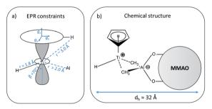
Scheme 1 (a) Summary of all constraints and structural parameters derived from the analysis of the EPR experiments (for clarity, only one out of the five Cp protons is shown), dashed lines represent trough–space interaction, whereas continuous lines represent direct bonds; (b) chemical structure derived from the EPR data, dashed lines represent the ion pair interaction between the [CpTi(III)] cation and the MMAO anion. The hydrodynamic diameter  $(d_h)$  of the ion pair is also reported.
