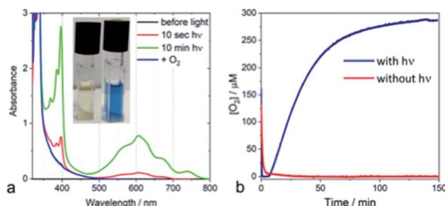
**Fig. 2** (a) Spectral changes induced in an Ar-purged solution of nano-PDPB,  $100 \mu\text{M } MV^{2+}$ , 10% TEOA in MeCN by illumination with blue light and after aeration (inset: formation of the blue  $MV^{+•}$  radical). (b) Time courses of oxygen evolution from water measured by a Clark electrode. Blue curve: with nano-PDPB (synthesized in mesophases) and red curve: no irradiation.
