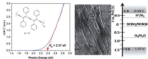
**Fig. 1** (Left) Tauc plot; middle: TEM image of nano-PDPB; and (right) energy diagram representing the evaluated valence band (V.B.) and conduction band (C.B.) levels of the PDPB polymer with regard to the water splitting reactions.
