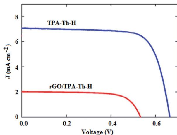
Fig. 7 *J*-*V* curves for the rGO/TPA-Th-H and TPA-Th-H-based DSSCs.<sup>119</sup>
