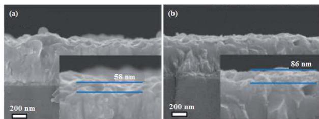
Fig. 10 Cross-sectional FE-SEM micrographs of (a) Pt and (b) Pt/rGO counter electrodes.<sup>186</sup>
