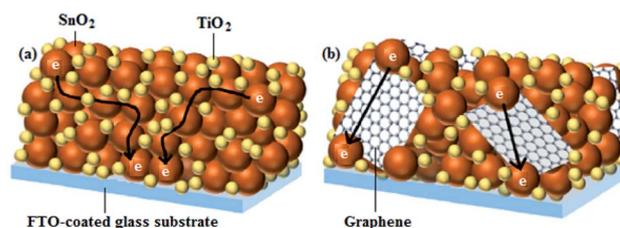
Fig. 6 An illustration of electron transport (a) in the TiO<sub>2</sub>/SnO<sub>2</sub>, and (b) TiO<sub>2</sub>/SnO<sub>2</sub>/graphene photoanodes.<sup>99</sup>
