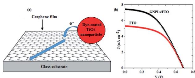
Fig. 4 (a) A schematic illustration of electron injection from a dye-coated  $\text{TiO}_2$  nanoparticle and transport in a continuous graphene film,<sup>65</sup> and (b) the  $J$ - $V$  characteristics of DSSCs based on GNPLs/FTO and pristine FTO electrodes.<sup>61</sup>
