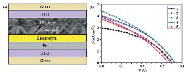
Fig. 5 (a) A schematic diagram of the GO/TiO<sub>2</sub>/Ag-based DSSC,<sup>84</sup> and (b) the  $J$ – $V$  characteristics of DSSCs based on: (1) ZnAl–MMO 8 : 1, (2) ZnAl–10 ml GO, (3) ZnAl–20 ml GO, (4) ZnAl–30 ml GO, and (5) ZnAl–40 ml GO, semiconducting layers.<sup>85</sup>
