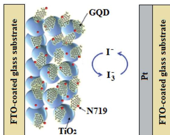
Fig. 8 A schematic diagram of the GQD/N719-based DSSC.<sup>129</sup>
