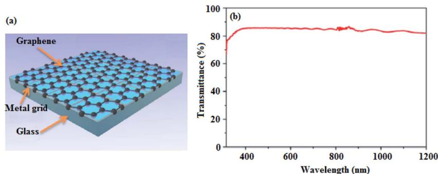
Fig. 3 (a) The hybrid graphene/metal grid transparent conducting electrode, and (b) the optical transmittance spectrum of the graphene/Ni electrode.<sup>59</sup>
