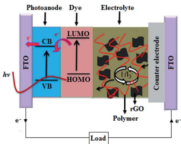
Fig. 9 A schematic diagram of the rGO/polymer-based DSSC.<sup>159</sup>
