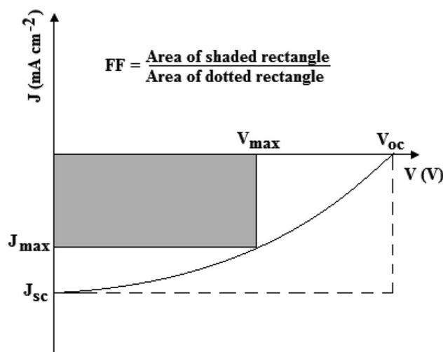
Fig. 2 A typical  $J$ – $V$  curve for an illuminated DSSC.
