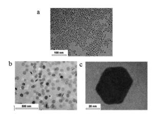
Fig. 4 (a) TEM images of the 5 nm GQDs distributed in methanol. (b and c) High resolution and low magnification pictures of the 70 nm size GQDs in methanol. Reprinted with permission.<sup>85</sup> Copyright 2019, American Chemical Society.
