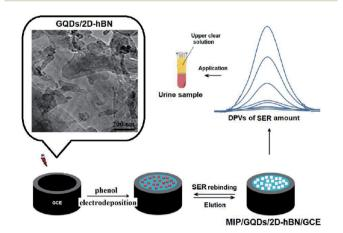
Fig. 9 MIP/GQDs/2D-hBN/GCE process. Reprinted with permission. 148 Copyright 2018, Elsevier.
