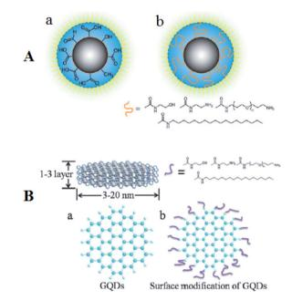
**Fig. 3** (A) Depiction of C-dots (a) following the treatment of surface oxidative and (b) following functionalizing with the surface-passivation reagent. (B) (a) A schema of the GQDs and (b) structural patterns following the functionalization with the surface-passivation reagents. Reprinted with permission. Copyright 2006, American Chemical Society.
