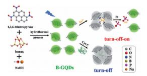
Fig. 2 A schema of the one-phase procurement of the B-GQDs to make the sensors (toward the Fe<sup>3+</sup> ion and phosphate-Pi) as well as the bio-sensor (toward the cytochrome C-Cyt C). Reprinted with permission.<sup>74</sup> Copyright 2019, Elsevier.
