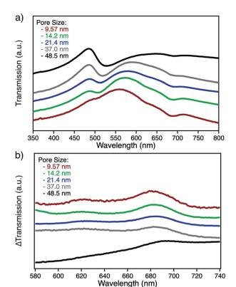
Fig. 5 (a) UV-Vis transmission spectra of ZnPc functionalized npAu foils in a DMF surrounding environment after dealloying times of 15 min (red), 30 min (green), 2 h (blue), 8 h (grey) and 72 h (black) and (b) Differential spectra of functionalized and unfunctionalized npAu foils showing the absorption of the immobilized ZnPc derivative 2.
