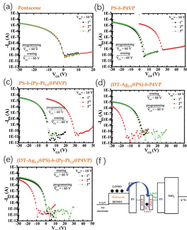
**Fig. 10**  $V_{th}$  shifts in the transfer characteristics of the devices incorporating (a) bare SiO<sub>2</sub>, (b) PS-*b*-P4VP, (c) PS-*b*-(Py-Pt<sub>1.0</sub>@P4VP), (d) (DT-Ag<sub>1.0</sub>@PS)-*b*-P4VP, and (e) (DT-Ag<sub>1.0</sub>@PS)-*b*-(Py-Pt<sub>1.0</sub>@P4VP). (f) Schematic diagram of the carrier tunnelling through the polymer electret into the metal NPs. Reproduced with permission.<sup>57</sup> Copyright 2013, Royal Society of Chemistry.
