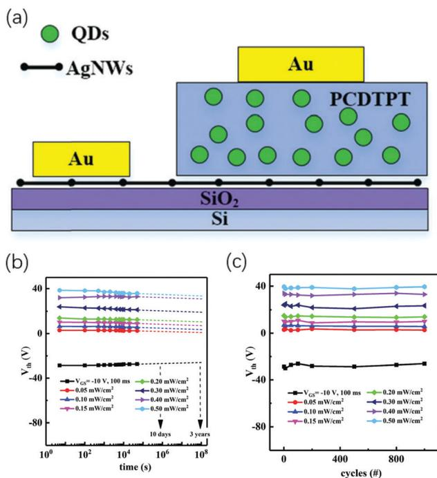
Fig. 16 (a) Schematic illustration of the photonic memory transistor. The retention curves of  $V_{th}$  (b) and the endurance curves of  $V_{th}$  (c) of photonic memory devices after light programming under light illumination (300 nm) with different light intensities for 0.5 s and after electric erasing with gate bias  $V_G = -10$  V for 100 ms. Reproduced with permission.<sup>79</sup> Copyright 2020, Royal Society of Chemistry.
