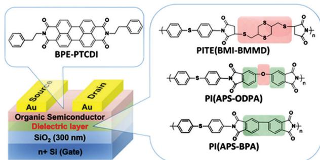
Fig. 7 Schematic diagram of the studied polymer electret OFET memory devices and the molecular structures of the studied PIs. Reproduced with permission.<sup>55</sup> Copyright 2014, John Wiley and Sons.
