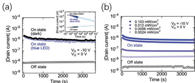
Fig. 15 (a) Retention curves of drain currents measured at  $V_G = 0$  V and  $V_D = -10$  V in the dark and under blue light illumination (469 nm,  $1.06 \text{ mW cm}^{-2}$ ) before and after programming with blue light. (b) Retention curves measured in the dark before and after programming ( $V_G = +60$  V, 3 s) with blue light at different intensities. Reproduced with permission.<sup>90</sup> Copyright 2019, Elsevier.
