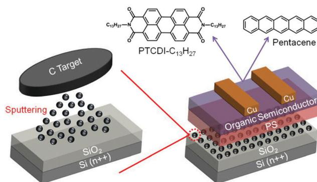
Fig. 4 Schematic representation of a pentacene-based or PTCDI- $\text{C}_{13}\text{H}_{27}$ -based floating gate OFET memory device (right), in which a PS layer and sputtered C-NPs (left) on top are employed as a tunnelling dielectric and nano floating gate, respectively. Reproduced with permission.<sup>41</sup> Copyright 2014, AIP Publishing.
