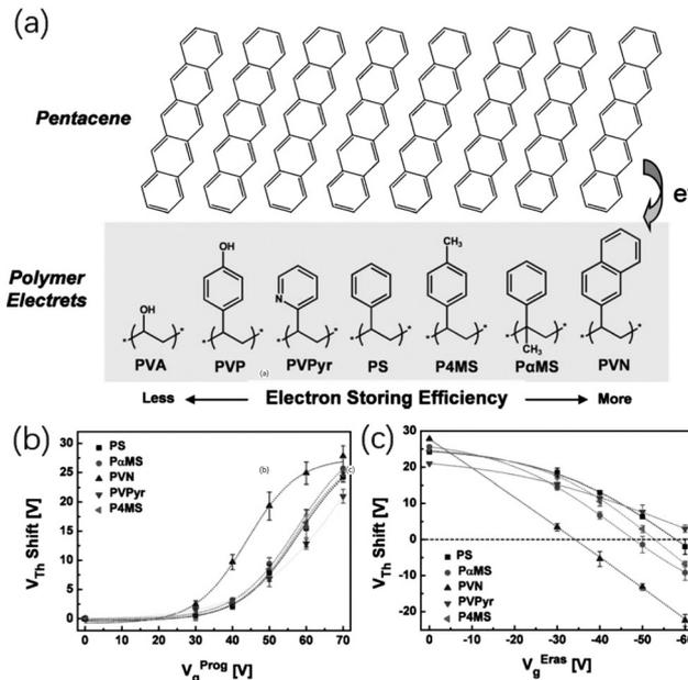
Fig. 6 (a) Schematic representation of the electron-storage efficiency of polymer electret materials estimated from the PEM characteristics. Shifts in  $V_{\text{th}}$  of PEM devices after the application of different gate biases during the (b) programming and (c) erasing processes. The dotted lines are fits to the measured points using a sigmoid function (Boltzmann fits). Reproduced with permission.<sup>51</sup> Copyright 2008, John Wiley and Sons.
