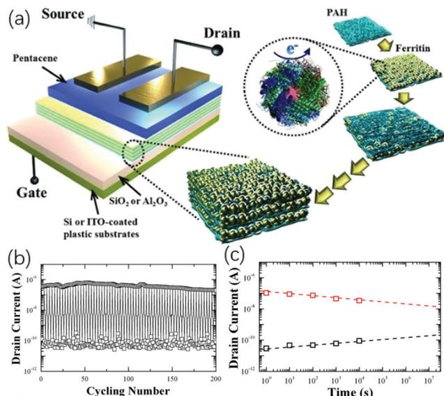
Fig. 3 (a) Schematic representation of the OFET memory device with LBL-assembled (PAH/ferritin NP)<sub>n</sub> multi-layered gate dielectrics. (b) Cycling and (c) retention time tests for devices with (PAH/ferritin NP)<sub>40</sub> multi-layers. Reproduced with permission.<sup>37</sup> Copyright 2013, John Wiley and Sons.
