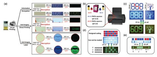
Fig. 21 (a) Potential applications of F-CD-based ink in information encryption, direct printing on a coupon, and Moutai Liquor anticounterfeiting tags. (b) Schematic illustrations of a representative customized tricolor inkjet cartridge. (c) Demonstration of lifetime encoding for security applications. Digital photographs of (d) binary-coded and (e) Morse-coded two-color microarray data storage chips. Reprinted from ref. 156 and 158 with permission. Copyright (2018) Wiley-VCH.
