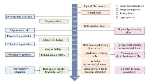
Fig. 97 Advances in fiber electronic devices with four main functions: energy harvesting, energy storing, sensing, and lighting according to the timeline.
