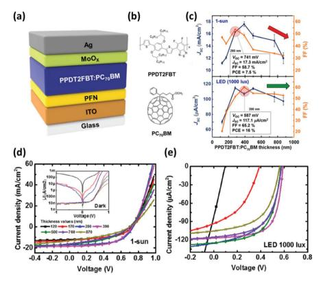
Fig. 5 Active layer thickness effect under 1 sun and LED illumination. (a) The device architecture and (b) molecular structures of PPDT2FBT and  $PC_{71}BM$ . (c) Active layer thickness dependent  $J_{SC}$  and FF under 1 sun and LED illumination. J-V characteristics with various photoactive layer thicknesses under (d) AM 1.5G and (e) LED (1000 lx) illumination. (Inset of (d): dark J-V curves.) Reproduced from ref. 47 with permission from Elsevier.
