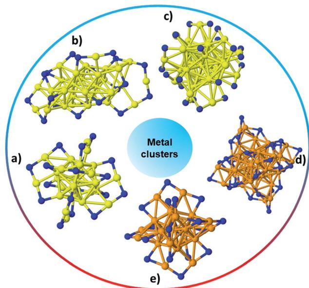
Fig. 1 The structure of (a)  $\text{Au}_{25}(\text{SR})_{18}$ ,<sup>35</sup> (b)  $\text{Au}_{30}\text{S}(\text{SR})_{18}$ ,<sup>36</sup> (c)  $\text{Au}_{38}(\text{SR})_{24}$ ,<sup>37</sup> (d)  $\text{Ag}_{44}(\text{SR})_{30}$ ,<sup>40</sup> (e)  $\text{Ag}_{25}(\text{SR})_{18}$ .<sup>38</sup> Au: yellow, S: blue, and Ag: orange. Only the S atoms of thiolates are shown while the rest of the ligand has been omitted for clarity.
