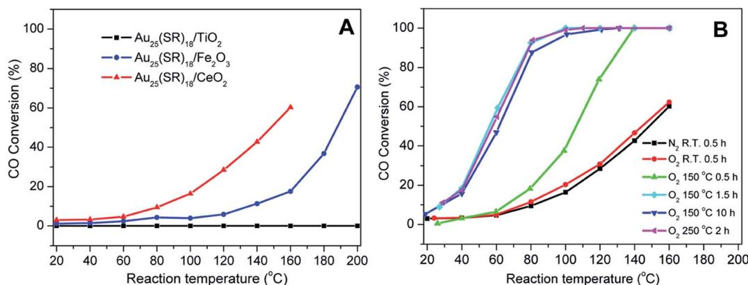
Fig. 3 Activation of  $\text{Au}_{25}(\text{SR})_{18}$  clusters over different metal oxides for CO oxidation. (A) CO activity over different metal oxides as a function of temperature for unactivated clusters, and (B) CO activity on ceria supports under different activation conditions. Reprinted with permission from ref. 49. Copyright 2012, American Chemical Society.
