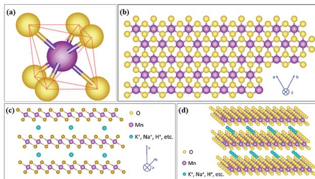
Fig. 1 (a)  $MnO_6$  octahedron unit; (b) schematic diagram of birnessite along the 001 plane; (c) schematic diagram of birnessite viewed along the 011 plane; (d) stereoscopic schematic diagram of birnessite.
