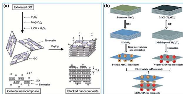
Fig. 14 (a) Schematic representation of GO–birnessite nanocomposites.<sup>169</sup> (b) Illustration of the process of preparing the birnessite/MXene composite.<sup>170</sup>
