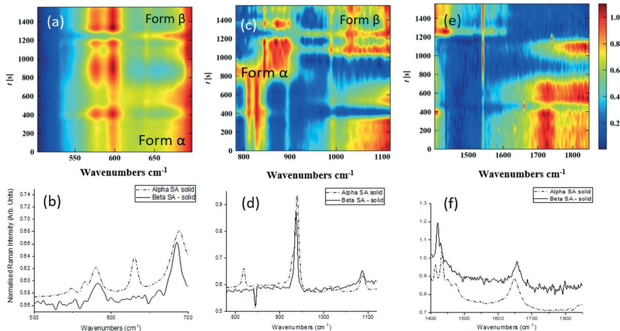
Fig. 4 Time-dependent Raman spectra collected from pre-prepared high density slurry of succinic acid form  $\alpha$ . In the region of (a) 500–700  $\text{cm}^{-1}$ , (b) corresponding 1D spectrum (c) 780–1120  $\text{cm}^{-1}$ , (d) corresponding 1D spectrum (e) 1400–1850  $\text{cm}^{-1}$ , (f) corresponding 1D spectrum. The regions of interest were scaled individually, to enhance the Raman peaks from the solids flowing through.
