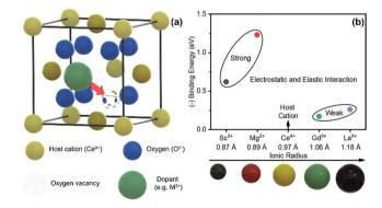
Fig. 1 (a) Schamatic illustration of a unit cell of fluorite structured ceria, showing electrosteric interaction between the acceptor dopant and charge compensating oxygen vacancy. (b) Computationally calculated binding energy (1nn) values of variously doped ceria as a function of dopant radius. The data are taken from V. Butler et al. 24
