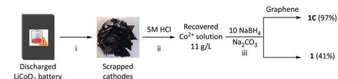
Scheme 2 Preparation sequence for **1** and **1C**. (i) Manual dismantling and separation of cathode materials. (ii) Dissolution in 5 M HCl at 80 °C for 1 h. (iii) neutralisation and treatment with 10 eq. of NaBH<sub>4</sub> in ethanol, in the presence or absence of graphene.
