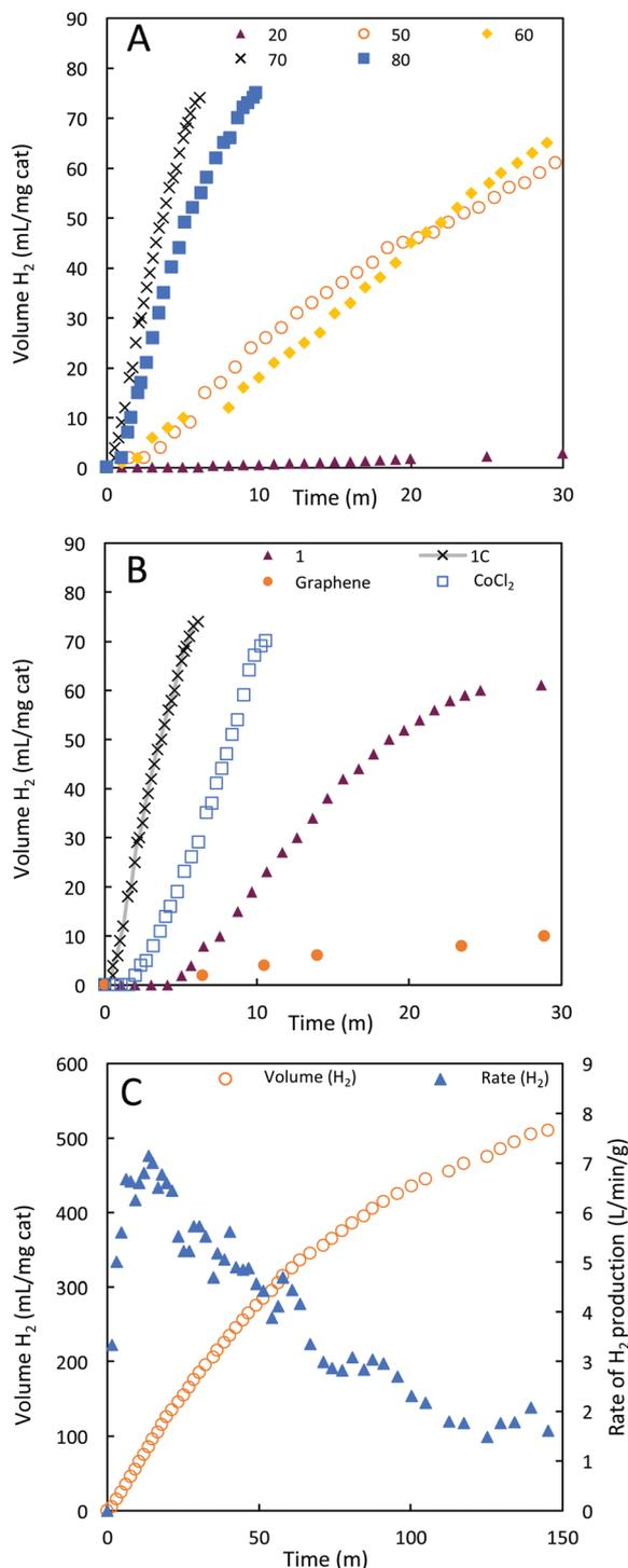
**Fig. 6** (A) Hydrogen production by 1 mg of **1C** at different temperatures from a 0.25 M NaBH<sub>4</sub><sup>-</sup> solution. (B) Hydrogen production of **1C**, **1** and graphene at 70 °C from a 0.25 M NaBH<sub>4</sub><sup>-</sup> solution. (C) Larger scale H<sub>2</sub> evolution experiment at 70 °C using 1 mg of **1C**, the blue triangles indicate the rate of hydrogen production over time, and the orange circles indicate the cumulative volume produced.
