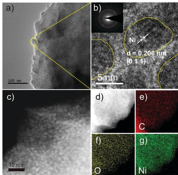
**Fig. 2** (a) TEM image; (b) HRTEM image and SAED pattern (inset); (c) STEM image of Ni NPs/C@Ni-MOF-74/NF(18 h); (d) HAADF-STEM image; (e–g) elemental mapping images of Ni NPs/C@Ni-MOF-74/NF(18 h), revealing the homogeneous distributions of C, O, and Ni elements.
