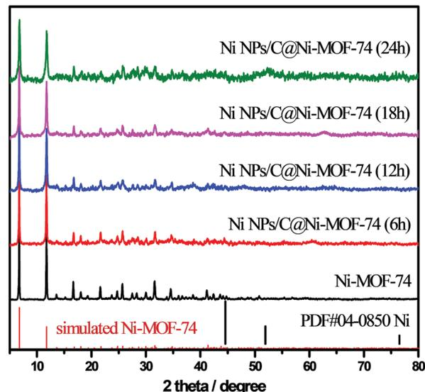
Fig. 1 PXRD patterns of Ni-MOF-74 and various Ni NPs/C@Ni-MOF-74 samples, and the simulated XRD patterns of Ni-MOF-74 (red bar) and metal Ni (black bar).
