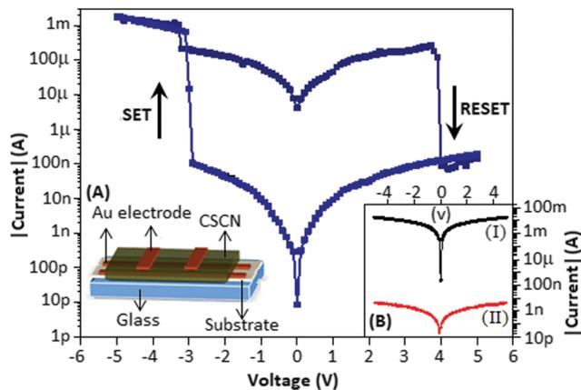
Fig. 3 Semi-log current-voltage ( $I$ - $V$ ) characteristics of the DUT, Au||CSCN||Au is bipolar in nature (main panel). Inset (A): Cross-bar structure of the Au||CSCN||Au device. Inset (B): Semi-log  $I$ - $V$  of 0.5:5 and 2:5 of copper nitrate to thiourea (by wt) compositions.
