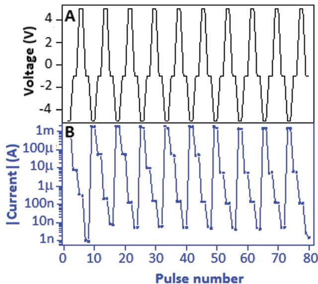
Fig. 7 (A) The Write–Read (1)–Erase–Read (0) voltage cycle ( $-5.0$ ,  $-1.0$ ,  $+5.0$  and  $-1.0$  V) applied to the device and (B) the respective current response (semi-log scale) received from the device.
