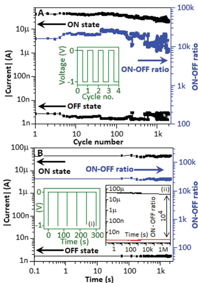
Fig. 6 (A) The endurance study of the device for  $2 \times 10^3$  cycles. The pulse train employed for the endurance study (inset). (B) The nonvolatile study of the device for  $2 \times 10^3$  s. The pulse train employed for the nonvolatile study with a duty cycle of 0.16%, inset (i). The estimated retention of the device after  $10^7$  s, inset (ii).
