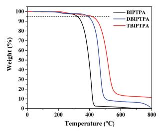
Fig. 1 Thermogravimetric curves of the luminophores.
