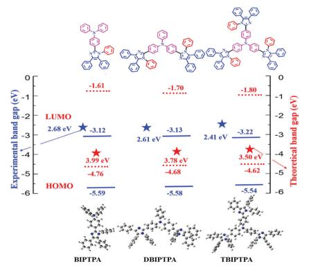
Fig. 7 HOMO-LUMO energy gap diagram of BIPTPA, DBIPTPA, and TBIPTPA luminophores.
