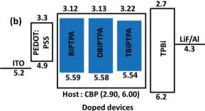
Fig. 8 Schematic representation of the energy levels of the solutionprocessed OLEDs composed of deep-blue BIPTPA, DBIPTPA and TBIPTPA emitters (a) undoped and (b) doped in CBP host devices.
