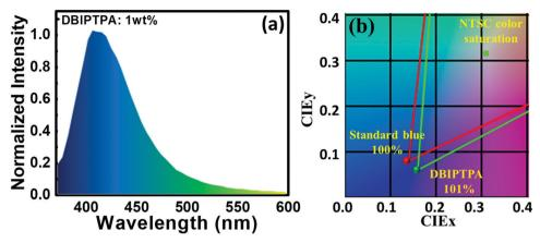
Fig. 12 (a and b) EL spectrum and NTSC color saturation of the solution-processed OLEDs containing 1 wt% DBIPTPA as the emitter at the brightness of 100 cd m<sup>-2</sup>, respectively.
