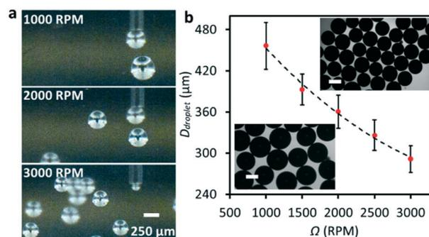
**Fig. 4** Production of EGaIn microdroplets using the RNEG. a) Images taken from a high-speed camera showing the production of liquid metal microdroplets at different revolving speeds. b) Plot of the droplet diameter  $D_{\text{droplet}}$  vs.  $\Omega$ . The inset images show the EGaIn droplets produced when  $\Omega$  is 1500 and 3000 rpm, respectively, and  $Q$  is  $20 \mu\text{L min}^{-1}$ .
