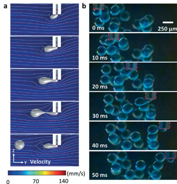
**Fig. 2** Droplet formation process. a) Numerical simulation results of the droplet breakup process at the needle tip. b) Sequential snapshots showing the formation of aqueous microdroplets using the RNEG (red dashed area is the needle tip and it moves from left to right).
