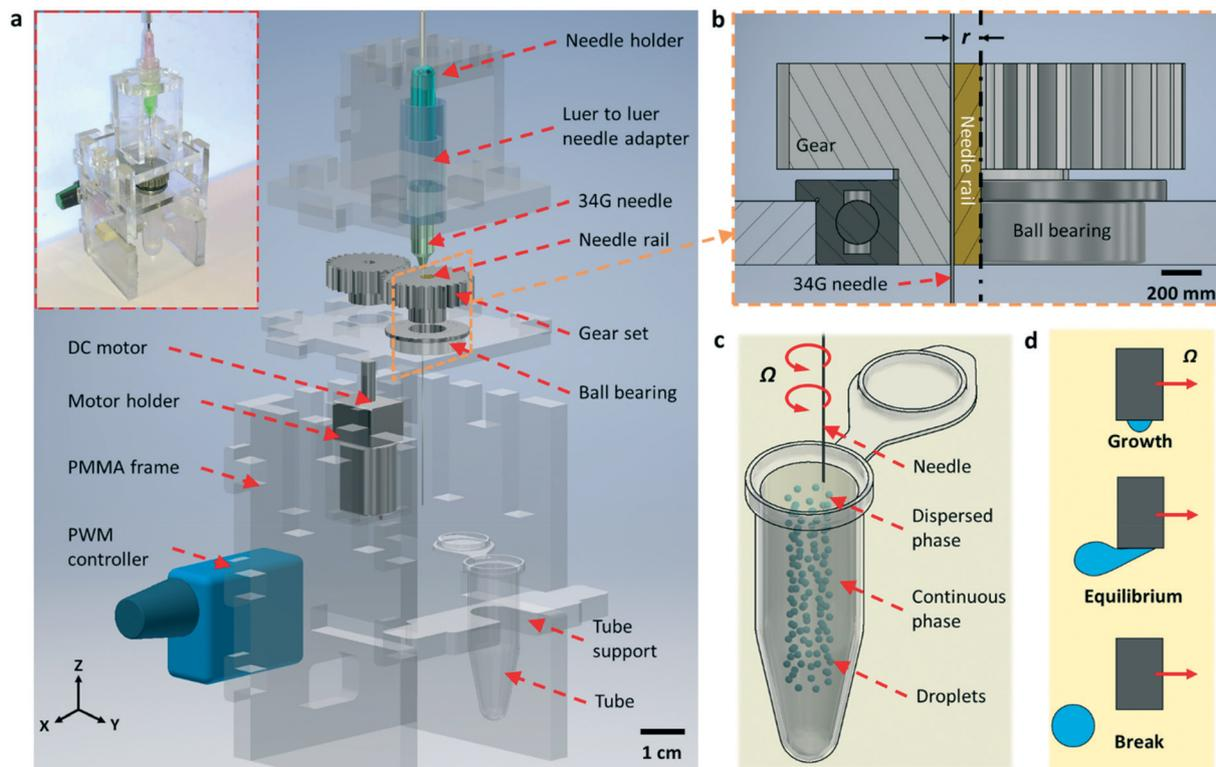
**Fig. 1** Schematic illustration of the revolving needle emulsion generator (RNEG). a) Exploded schematic representation of the RNEG. The upper inset shows an actual image of the assembled system. b) Zoomed-in schematic representation of the off-axis eccentric setup. c) Illustration of the generated microdroplets in a test tube. d) Schematics of the droplet formation process.
