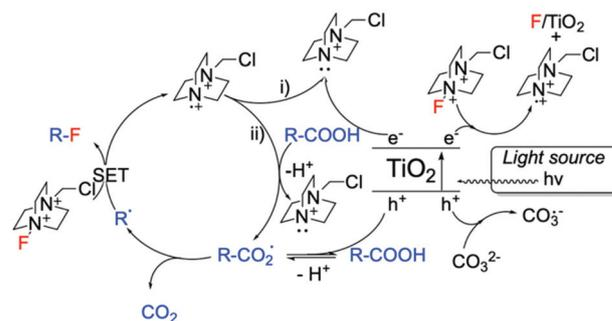
**Scheme 15** Proposed reaction mechanism for TiO<sub>2</sub>-photocatalysed decarboxylative fluorinations.<sup>102</sup> Scheme adapted with permission from ref. 102 (American Chemical Society, <https://pubs.acs.org/doi/10.1021/acscatal.8b02844>).
