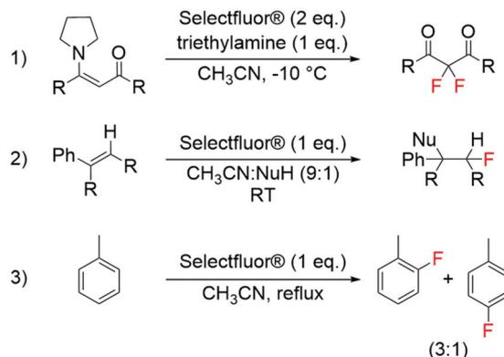
**Scheme 3** Examples of electrophilic fluorination reactions using Selectfluor®: (1) synthesis of difluorinated carbonyl compounds from enamines,<sup>58</sup> (2) fluorination of alkenes,<sup>59</sup> and (3) synthesis of aryl fluorides from aromatic compounds.<sup>59</sup>
