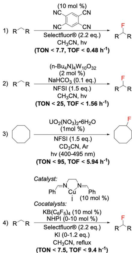
**Scheme 13** Examples of photocatalytic aliphatic fluorinations reported by: (1) Bloom *et al.*<sup>126</sup> (2) Halperin *et al.*<sup>127</sup> (3) West *et al.*<sup>128</sup> and (4) Cu-initiated radical aliphatic fluorination reported by Bloom *et al.*<sup>107</sup>
