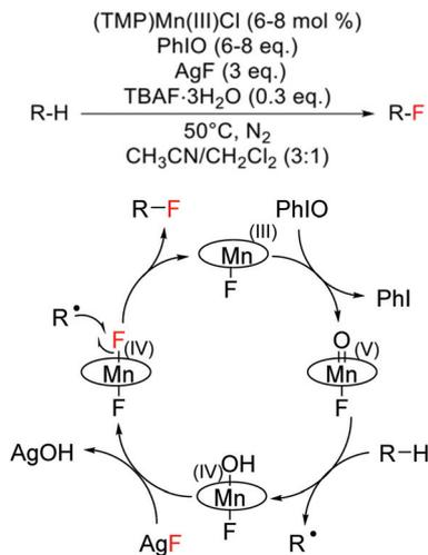
**Scheme 12** Reaction scheme and proposed reaction mechanism for direct alkane fluorination catalysed by a Mn(III)-porphyrin.<sup>119</sup> Reaction scheme adapted from ref. 119.
