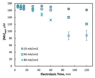
Fig. 2 Removal of aqueous manganese (Mn²+) with electrolysis time and current densities of 10, 40 and 80 mA cm²-2 (pH = 7, [Mn²+] $_0$  = 175  $\mu$ M, T = 21.0  $\pm$  0.8 °C).
