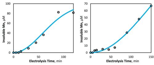
Fig. 7 Model and experimentally yielded results of insoluble manganese (Mn<sup>3+,4+</sup>) generation at 80 mA cm<sup>-2</sup> (left) and 40 mA cm<sup>-2</sup> (right) (pH = 7, [Mn<sup>2+</sup>]<sub>0</sub> = 175  $\mu$ M, T = 21.0  $\pm$  0.8 °C).
