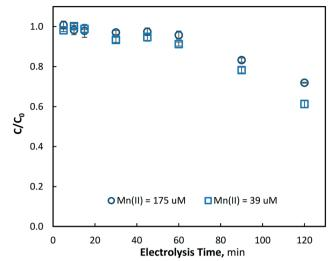
Fig. 6 Removal of aqueous manganese (Mn<sup>2+</sup>) with electrolysis time at 40 mA cm<sup>-2</sup> with [Mn<sup>2+</sup>]<sub>0</sub> = 175 and 39  $\mu$ M, (pH = 7, T = 21.0  $\pm$  0.8 °C).
