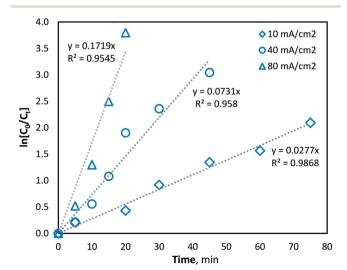
Fig. 4 Indirect quantification of hydroxyl radical formation (methanol degradation) with current densities of 10, 40 and 80 mA cm $^{-2}$  (pH = 7, T = 21.0  $\pm$  0.8 °C).
