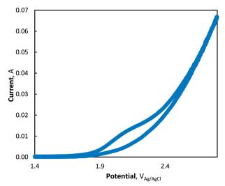
Fig. 3 Cyclic voltammogram of  $MnCl_2$  at pH = 7 (phosphate buffer) and 10 mV s<sup>-1</sup> scan rate.
