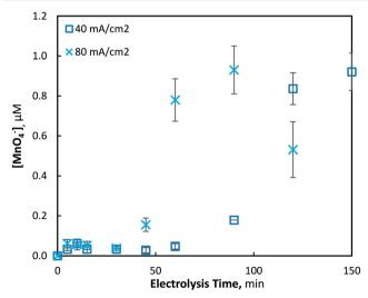
Fig. 8 Production of permanganate at 40 and 80 mA cm $^{-2}$  over 120 min of electrolysis (pH = 7, [Mn $^{2+}$ ] $_0$  = 175  $\mu$ M, T = 21.0  $\pm$  0.8  $^{\circ}$ C).
