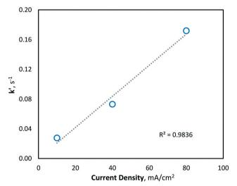
Fig. 5 Pseudo-first-order rate constant (k') of MeOH degradation via hydroxyl radical oxidation at various current density conditions (10, 40 and 80 mA cm<sup>-2</sup>).
