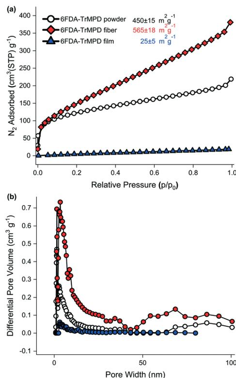
**Fig. 4** a) Nitrogen adsorption isotherms measured at  $-196 \text{ }^\circ\text{C}$  up to 1 bar, b) NLDFT-derived pore size distributions of the 6FDA-TrMPD polymer powder, the nanofibrous mat and the film.
