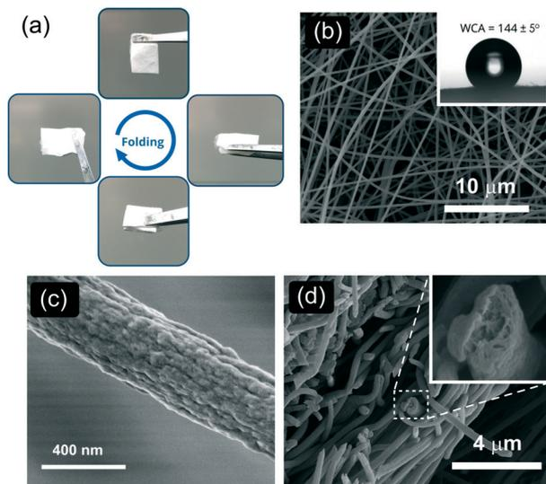
**Fig. 2** (a) Optical photos showing the 6FDA-TrMPD mat during the folding/unfolding process,  $C_{6FDA-TrMPD} = 10\%$  (w/v). (b) SEM image of the nanofibers and its water wettability showing hydrophobicity. (c) SEM image of a single nanofiber showing a wrinkled texture. (d) Cross-section image of the mat and fiber (inset).
