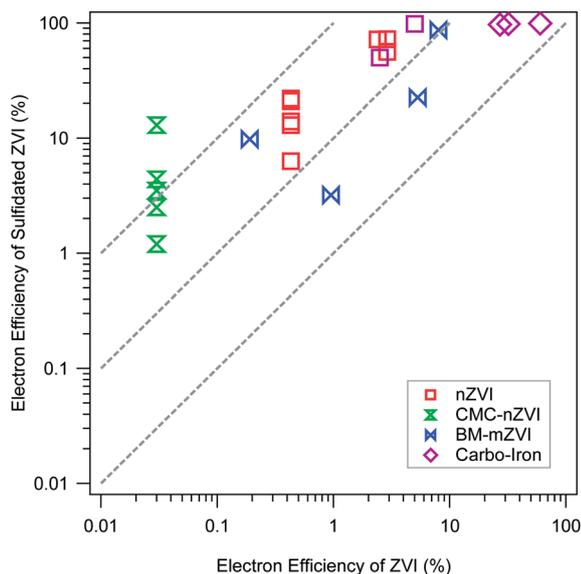
Fig. 4 Comparison of electron efficiencies ( $\epsilon_e$ ) for TCE reduction by ZVI with (*y*-axis) and without (*x*-axis) sulfidation. Types of ZVI are distinguished by the marker type and color. Data and experimental details are given in Table S1.†
