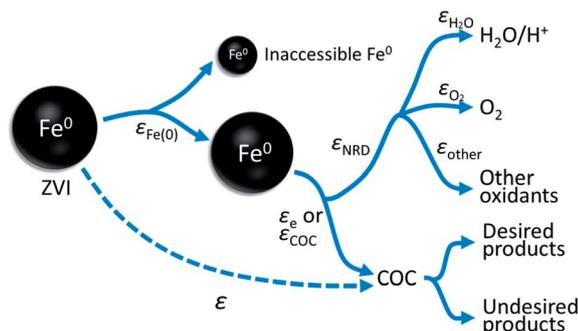
Fig. 1 Summary of the relationship between the particle efficiency ( $\epsilon$ ), efficiency of Fe(0) utilization ( $\epsilon_{\text{Fe}(0)}$ ), electron efficiency ( $\epsilon_e$  or EE) of contaminant reduction, and the electron efficiency of NRD (e.g., H<sub>2</sub>O, O<sub>2</sub>, and other oxidants) reduction ( $\epsilon_{\text{NRD}}$ ). Earlier versions of this conceptual model can be found in Qin *et al.*<sup>15</sup>
