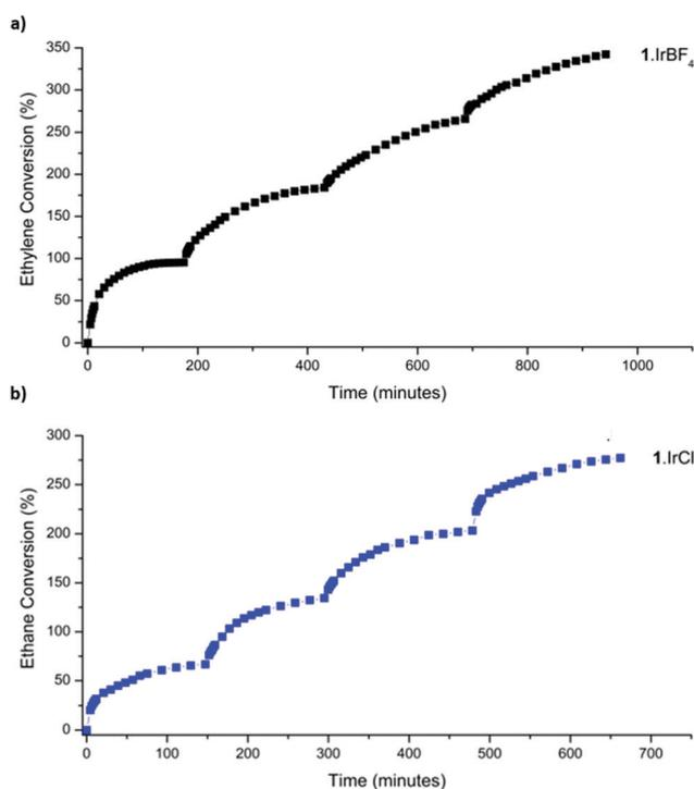
Fig. 3 Catalysis data for the hydrogenation of ethylene at 46 °C (2 bar) using (a) **1**-IrBF<sub>4</sub> and (b) **1**-IrCl.
