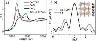
Fig. 2 (a) XANES spectra of Ce-TCPP MOFs (red), CeCl<sub>3</sub> (blue), CeO<sub>2</sub> (black) and (NH<sub>4</sub>)<sub>2</sub>Ce(NO<sub>3</sub>)<sub>6</sub> (olive). (b) The Fourier-transformed XAS spectrum of Ce-TCPP in R-space. The inset shows the fitting model. The data are shown as open dots and FEFF fits are shown as solid lines.
