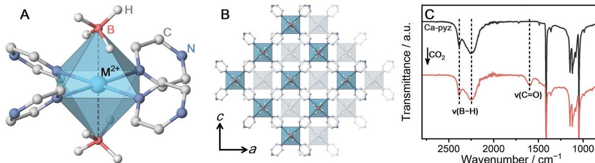
Fig. 1 (A) Local coordination geometry of **M-pyz** ( $M = \text{Mg}^{2+}, \text{Ca}^{2+}, \text{Mn}^{2+}$ ). (B) ABAB stacking structure of the extended 2D layers of **M-pyz** ( $M = \text{Mg}^{2+}, \text{Ca}^{2+}, \text{Mn}^{2+}$ ). (C) IR spectra of **Ca-pyz** before and after CO<sub>2</sub> adsorption at 25 °C.
