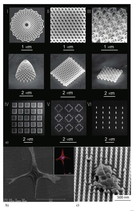
Fig. 5 (a) Some examples of the nanofeatures created on the surface of origami-based meta-biomaterials using EBID.<sup>104</sup> (b) The response of preosteoblast to nanopatterned surfaces. (c) Staphylococcus aureus can be killed by nanopatterns. 95
