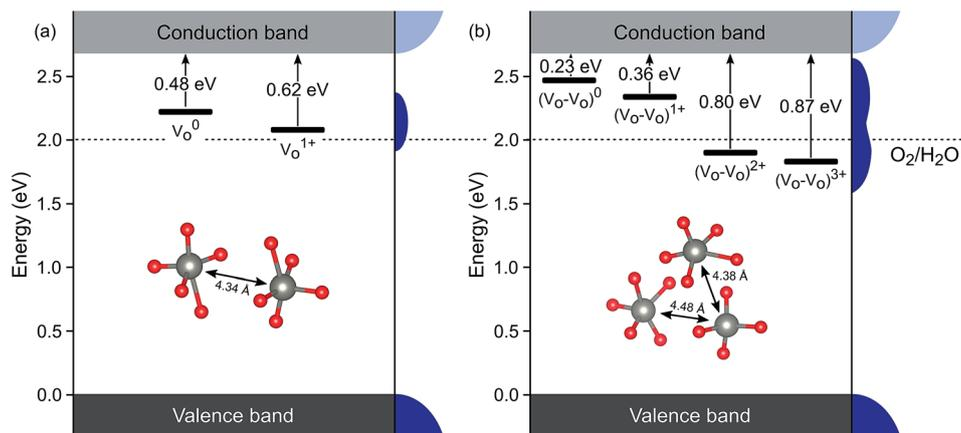
Fig. 3 Defect ionisation levels of oxygen vacancies in different charge states calculated from hybrid density functional theory for (a) an isolated oxygen vacancy  $V_{\text{O}}(y)$  and (b) a defect complex composed of two oxygen vacancies  $V_{\text{O}}(z)$ . Energies are relative to the valence band edge. Densities of states are illustrated schematically at the right side of each panel. The insets show local atomic structures and the distance between the W atoms.
