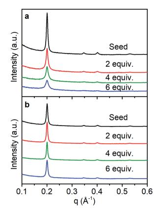
Fig. 5 WAXS diffraction monitoring change in crystallinity as monomers are added with a rate of (a) 50 equiv.  $h^{-1}$ , (b) 1 equiv.  $h^{-1}$ .
