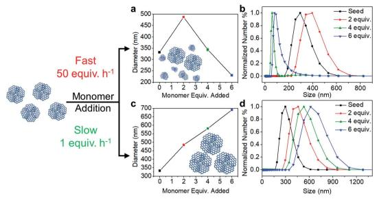
Fig. 3 Trend in the average size of particles with monomer addition at a fast rate of 50 equiv.  $h^{-1}$  and at a slow rate of 1 equiv.  $h^{-1}$ . (a, c) Average size of particles with additional equivalents of monomers (b, d) corresponding number percent distribution.
