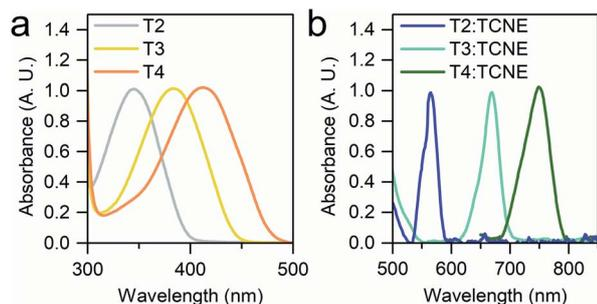
Fig. 2 UV-vis spectra of the T2–T4 series (a) and of their TCNE complexes (b) in  $\text{CH}_2\text{Cl}_2$ . A 1 : 100 ratio of molecule : TCNE was used to obtain (b). All the spectra are normalised, and the onset of the T4  $\pi \rightarrow \pi^*$  band below 650 nm in (b) was removed for clarity. The CT bands are two orders of magnitude less intense than the  $\pi \rightarrow \pi^*$  transition.
