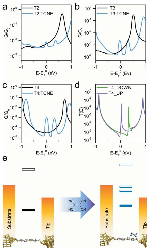
**Fig. 4** Room temperature calculated conductance for the isolated molecules (black line) and complexed with TCNE (blue) for compounds T2 (a), T3 (b) and T4 (c), along with a representative spin-polarised  $T(E)$  curve for the TCNE complex of T4 (d). Schematic diagram (e) showing the position of the DFT resonances for T4 relative to the two electrodes before and after TCNE complexation. The part-filled CT resonances in the HOMO–LUMO gap are responsible for the observed increase in conductance.
