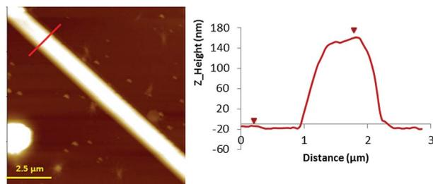
Fig. 3 Left: AFM Z-height images of microcrystals **2** prepared on a Si/SiO<sub>2</sub> substrate. Right: line profile for height.
