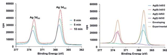
Fig. 4 Left: High resolution XPS spectrum of the Ag3d region for compound **2** before and after exposure to cold hydrogen plasma. Right: The experimental data (orange line) was fitted (dash line) to the sum of the 3d<sub>5/2</sub> and 3d<sub>3/2</sub> contributions of Ag<sup>0</sup> (blue and red lines, respectively) and Ag<sup>I</sup> (green and purple lines, respectively). The inset legend gives the time period of exposure to the hydrogen plasma.
