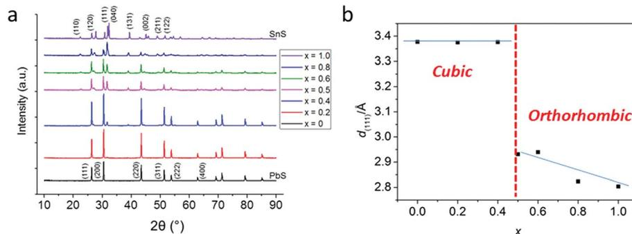
**Fig. 2** pXRD analysis of bulk  $\text{Pb}_{1-x}\text{Sn}_x\text{S}$  ( $0 \leq x \leq 1$ ) alloys. (a) Offset diffraction patterns of bulk  $\text{Pb}_{1-x}\text{Sn}_x\text{S}$  ( $0 \leq x \leq 1$ ) with major  $(hkl)$  reflections labelled. (b) Analysis of the  $d_{111}$  spacing as a function of compositional variation ( $x$ ). The red dash line shows the transition between cubic structures and orthorhombic structures.
