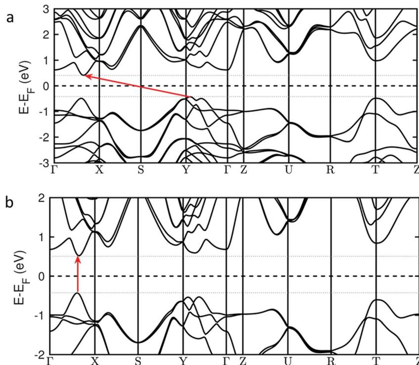
Fig. 11 Calculated band structures for bulk crystals of (a) SnS and (b) SnS in the  $\text{Pb}_{0.2}\text{Sn}_{0.8}\text{S}$  structure. The horizontal dashed lines show the Fermi energies and the red arrows the HOCO–LUCO excitations. HOCO (highest occupied crystal orbital) and LUCO (lowest unoccupied crystal orbital) are the edges of the valence and conduction bands respectively. The Fermi energy is set to zero.
