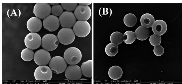
Fig. 2 SEM images of nanobowls formed from (A) PHAZoMA<sub>29</sub> and (B) PHAZoMA<sub>116</sub>.
