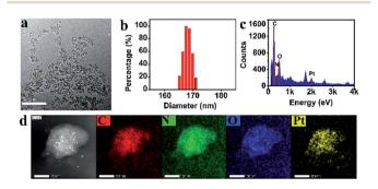
Fig. 1  $\,$  TEM ((a), scale bar 1  $\mu$ m), DLS (b), EDX (c), and STEM results and EDS elemental mapping of PCNH ((d), scale bar 100 nm).
