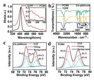
Fig. 2 Normalized UV-vis spectra of TCPP and PCNH ((a); the insert is the amplification figure of the Q bands). FT-IR spectra of TCPP, cisplatinum and PCNH (b). XPS fine spectra of cis-platinum (c) and PCNH (d)
