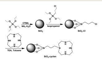
Scheme 1 Fabrication route to the SiO<sub>2</sub>-cyclen nanochelator.
