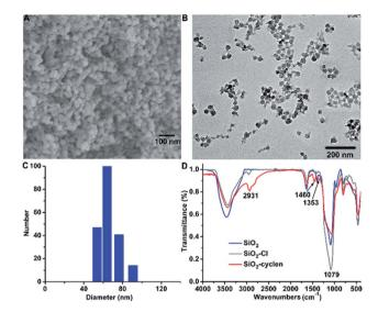
Fig. 1 SEM image (A), TEM image (B), DLS size distribution (C) of SiO $_2$ -cyclen nanochelator, and FT-IR spectra (KBr) of SiO $_2$ , SiO $_2$ -Cl and SiO $_2$ -cyclen (D).
