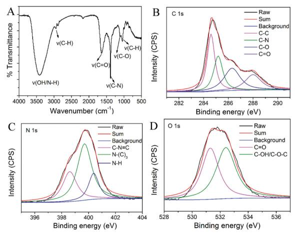
Fig. 2 (A) FT-IR spectrum of the N-dots. High resolution XPS spectra of (B) C 1s, (C) N 1s, and (D) O 1s peaks of the N-dots, respectively.
