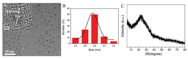
Fig. 1 The TEM and HRTEM (inset) images (A), the size distribution (B), and the powder XRD pattern (C) of the N-dots.
