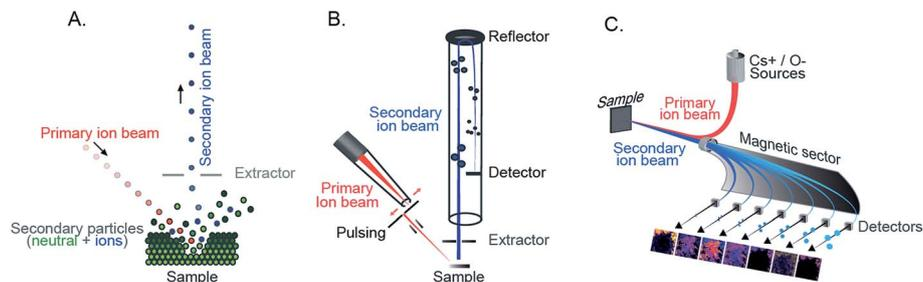
Fig. 1 (A) Principle of SIMS measurement. The primary ion beam sputters the sample surface producing secondary particles which include neutral particles and ions. The secondary ions are then extracted into the mass spectrometer. (B) Configuration of ToF-SIMS with a pulsed primary ion beam and a time-of-flight mass analyzer. (C) Configuration of nanoSIMS featuring the co-axial axis of the primary and secondary ion beams and a magnetic sector mass analyzer.
