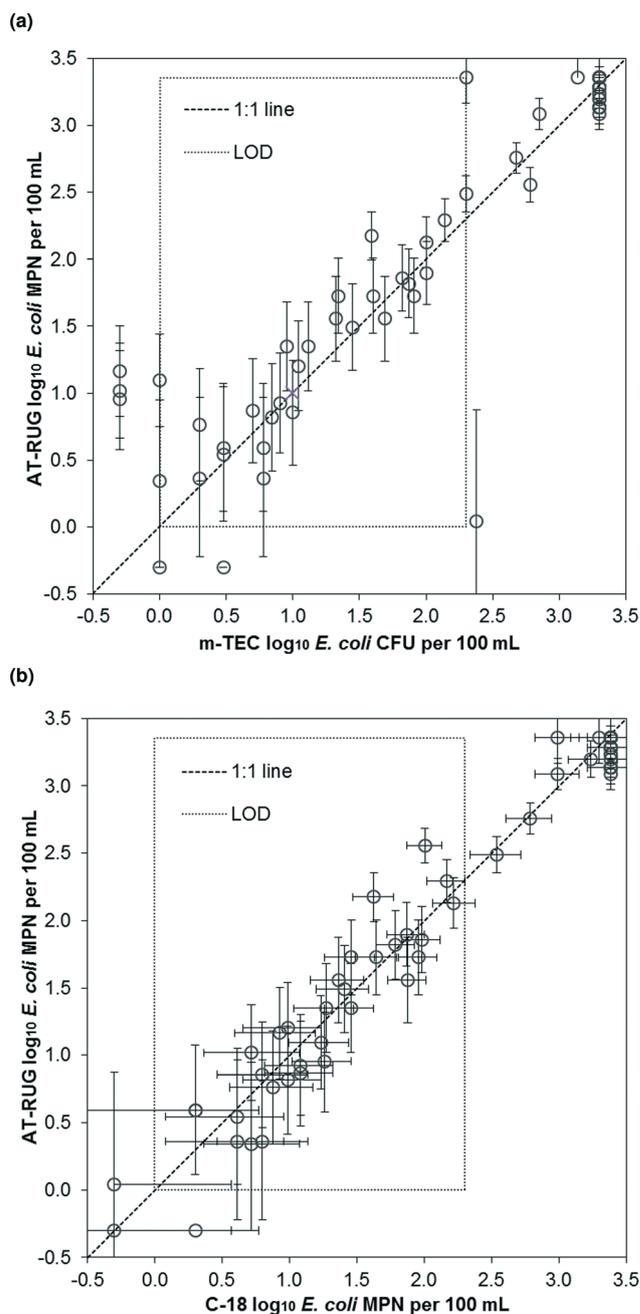
Fig. 2 Scatter plots of *E. coli* estimates using AT-RUG versus (a) m-TEC and (b) C-18. Error bars show the 95% confidence interval of the MPN assays for AT-RUG and C-18.
