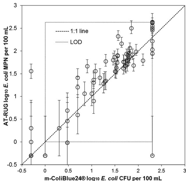
Fig. 3 Scatter plot of AT-RUG *E. coli* estimates with 95% confidence intervals versus m-ColiBlue24@. Confidence intervals are only valid in the range of detection.
