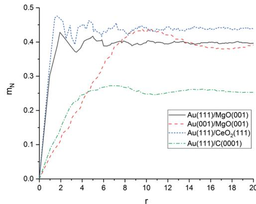
Fig. 6 Mismatch  $m_N(r)$  of Au on MgO, CeO<sub>2</sub> and C based on DFT surface calculations.
