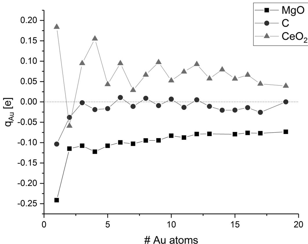
Fig. 8 Average charge of the gold atoms on MgO, C, and CeO<sub>2</sub>; values are connected to guide-the-eye.
