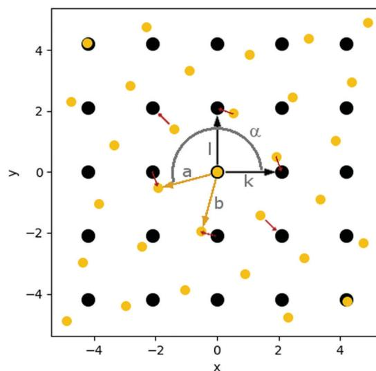
Fig. 4 Schematic representation of the grids of surface sites (black; defined by vectors  $k$  and  $l$ ) and cluster atoms (yellow; defined by vectors  $a$  and  $b$ ); angle  $\alpha$  defines rotation of cluster grid with respect to surface grid; local mismatch  $m_p$  at first neighbour atoms is represented with red arrows (see ESI† for more details on the mismatch calculation).
