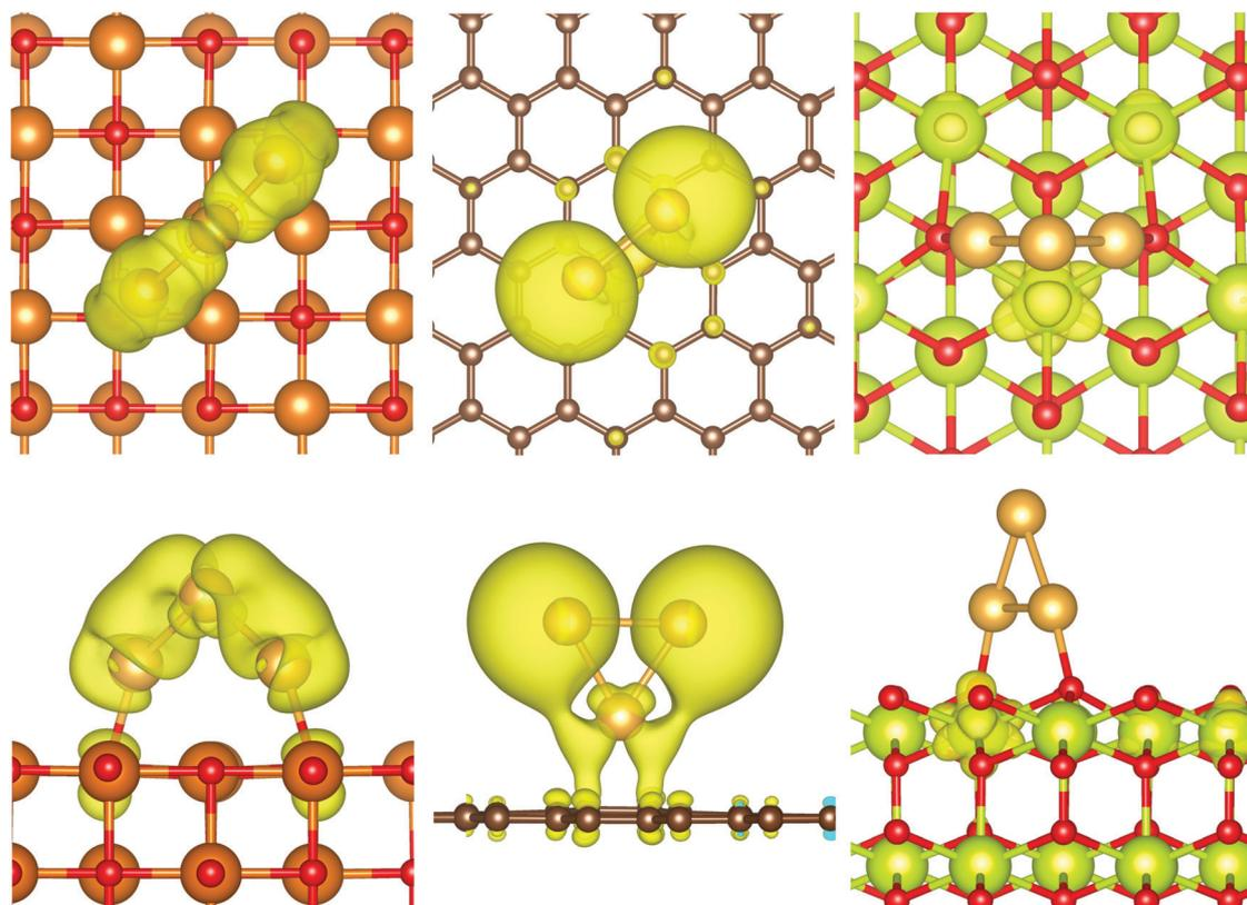
Fig. 9 Iso-surfaces of the highest occupied band of Au<sub>3</sub>/MgO (left), Au<sub>3</sub>/C (centre), and Au<sub>3</sub>/CeO<sub>2</sub> (right); iso-value of 0.001 e Å<sup>-3</sup>.
