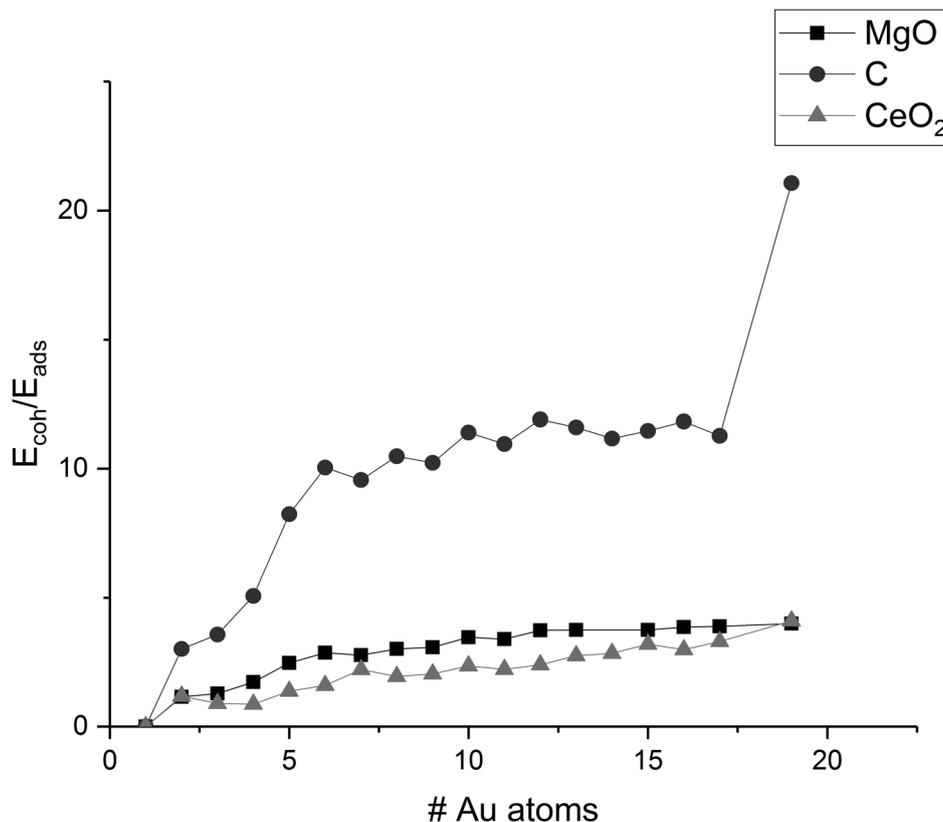
Fig. 5 Ratio of  $E_{\text{coh}}/E_{\text{ads}}$  of Au clusters on MgO, C, and CeO<sub>2</sub>; values are connected to guide-the-eye.
