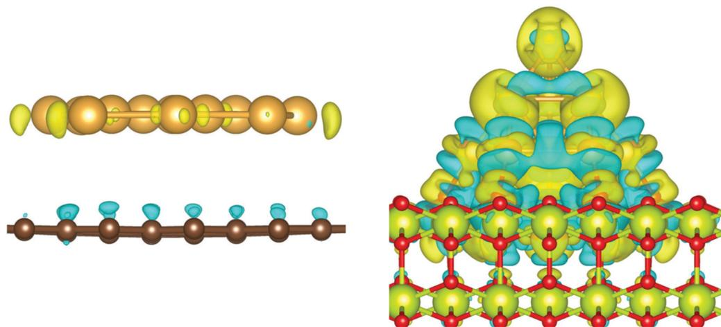
Fig. 7 Electron density flow of the adsorption of  $\text{Au}_{11}$  on graphene (left) and  $\text{CeO}_2$  (right) [ $\rho_{\text{Au-surface}} - (\rho_{\text{Au}} + \rho_{\text{surface}})$ ]; iso-value of  $0.001 e \text{ \AA}^{-3}$ ; positive values in yellow; negative values in turquoise.
