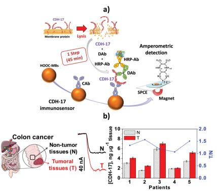
Fig. 15 (a) Schematic illustration of the immunosensor developed for CDH-17 determination. Illustrative examples of amperograms recorded with the immunosensor of  $0.5 \, \mu g$  of protein extracts obtained from a tumor (T) and paired healthy tissue (N), and CDH-17 concentrations obtained in the analyzed tissue extracts. Error bars are three times the standard deviation of three replicates. Reproduced and adapted from ref. 32 with permission.
