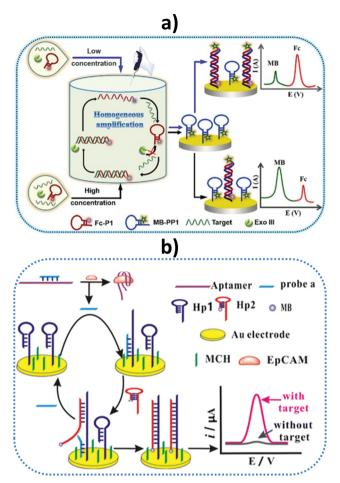
Fig. 10 Schematic illustrations of (a) a homogeneous Exo III-assisted target recycling amplification and dual-signal ratiometric electrochemical DNA biosensor, and (b) a sensor design and amplification strategy for the determination of epithelial cell adhesion molecule (EpCAM) and EpCAMdriven toehold-mediated DNA recycling amplification. MB, methylene blue; Fc, ferrocene; MCH, 6-mercapto-1-hexanol. Reproduced from (a) ref. 129 and (b) ref. 131 with permission.
