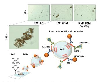
Fig. 14 Photomicrographs obtained for the sandwich immunoassays conducted with cell suspensions ( $1.0 \times 10^6 \, \text{cells mL}^{-1}$ ) on MBs unmodified and modified with the capture antibody (CAb). Reproduced and adapted from ref. 31 with permission.
