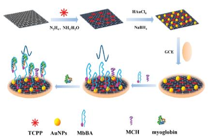
Fig. 2 Synthesis of TCPP-graphene/AuNP nanocomposites and an electrochemical aptasensor for myoglobin detection. Reproduced from ref. 96 with permission.
