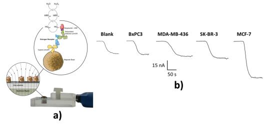
Fig. 13 (a) Schematic illustration of MB-based sandwich immunosensor developed for  $ER\alpha$  determination. (b) Amperometric responses recorded in the absence (blank) and presence of 2.5  $\mu g$  of raw lysates from the corresponding cells. Reproduced and adapted from ref. 53 with permission.
