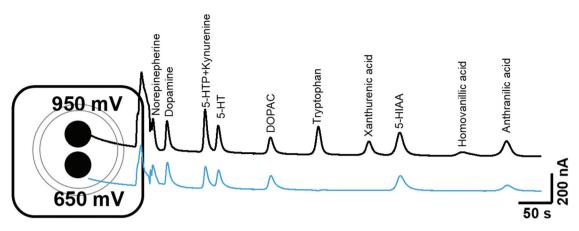
Fig. 2 Schematic of the dual glassy carbon electrode utilised for simultaneous detection of analytes at +950 mV and +650 mV. Dual voltage detection was utilised to aid separation and validation of analyte detection.
