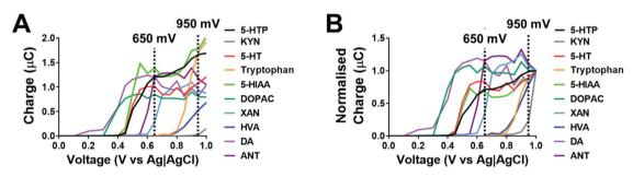
Fig. 3 Hydrodynamic voltammograms of all analytes. (A) shows the response of all analytes where the peak area was monitored every 50 mV from 1 V to 0 V. (B) The response of all analytes was normalised to the charge observed at 1 V in order to show the voltammetric profile of each analyte in a comparable fashion. The dashed line highlights the voltages of 950 mV and 650 mV, which were utilised for dual detection and separation of analytes.
