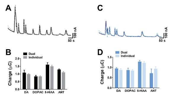
Fig. 5 Determination of crosstalk between dual electrodes. Measurements were performed at (A) +950 mV and (C) +650 mV, where the analyte mixture was injected when either both electrodes were held at the given potential (solid line) or an individual electrode was polarised (dashed line). The resultant peak areas from multiple runs at (B) 950 mV and (D) 650 mV show no difference between the dual electrode and individual electrode. Data shown as mean + standard deviation, n = 4.
