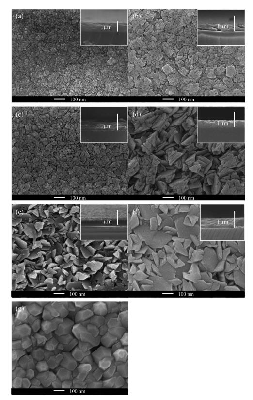
Fig. 6 SEM images of ZnO and Cl-doped ZnO films with mol% FeCl<sub>3</sub> loading of (a) 0 mol%, (b) 1 mol%, (c) 3 mol%, (d) 5 mol%, (e) 7 mol%, (f) 10 mol% and (g) 15 mol%. Side-on SEM (inset) shows film thickness.
