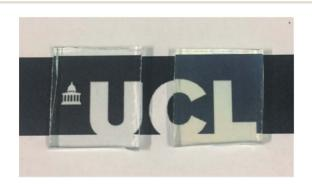
Fig. 2 Photograph of bare glass (left) and 7 mol% FeCl $_3$  loaded ZnO film (right).
