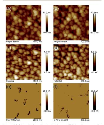
Fig. 4 (a), (c) and (e) are the height image, KPFM surface potential topology and photoconductive-AFM of the 2-Mo-BiVO $_4$  films; (b), (d) and (f) are the height image, KPFM surface potential topology and photoconductive AFM of the 2-Mo-BiVO $_4$  coated with the Fe-doped NiO catalyst. The surface potential was calibrated with an Au film (work function at 5.1  $\pm$  0.02 eV). The negative photocurrent in C-AFM corresponds to a positive charge flowing to the probe.
