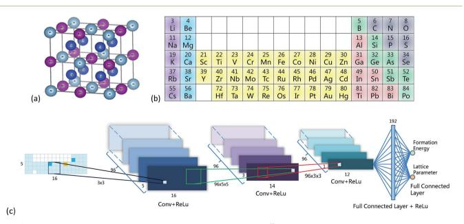
Fig. 1 (a) Crystal structure of an L2 $_1$  full-Heusler compound, created by using VESTA. $^{27}$  (b) Illustration of the periodic table representation. Colors were only guide for the eye, not used by the CNN. (c) Structure of the CNN.
