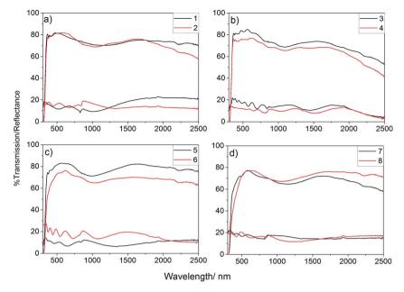
Fig. 4 UV/vis/NIR spectra for P-doped SnO<sub>2</sub> films; (a) undoped SnO<sub>2</sub> (1) and 0.1 mol% P:SnO<sub>2</sub> (2); (b) 0.25 mol% P:SnO<sub>2</sub> (3) and 0.5 mol% P:SnO<sub>2</sub> (4); (c) 1 mol% P:SnO<sub>2</sub> (5) and 1.5 mol% P:SnO<sub>2</sub> (6); and (d) 5 mol% P:SnO<sub>2</sub> (7) and 7.5 mol% P:SnO<sub>2</sub> (8). In all cases the films showed high transmission (ca. 80%) and low reflection (<20%). All films deposited by AACVD at 550 °C using air as carrier gas.
