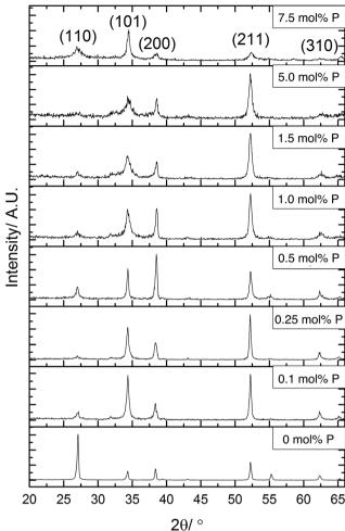
Fig. 2 X-ray diffraction patterns for  $P:SnO_2$  thin films deposited by AACVD at 550 °C. A change in preferred orientation is observed between undoped, and inclusion of phosphorus into the crystal structure.
