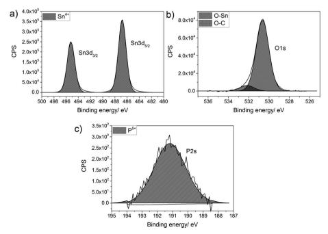
Fig. 1 Typical X-ray photoelectron spectra for (a) Sn 3d environment, (b) O 1s environment and (c) P 2s environment for P-doped SnO<sub>2</sub> films synthesised by AACVD at 550 °C.
