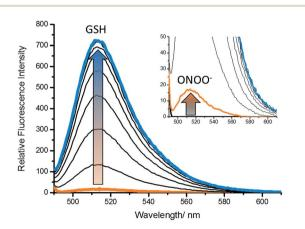
Fig. 1 Fluorescence spectra of GSH-PF3 (0.5  $\mu$ M) with addition of ONOO<sup>-</sup> (10  $\mu$ M) (inset) followed by the addition of GSH (0–80  $\mu$ M), 5 min wait between addition in buffer solution [52 wt% methanol] (pH = 8.21 at 25 °C). Fluorescence intensities were measured with  $\lambda_{ex}$  = 488 nm with slit widths ex slit: 5 nm and em slit: 2.5 nm.
